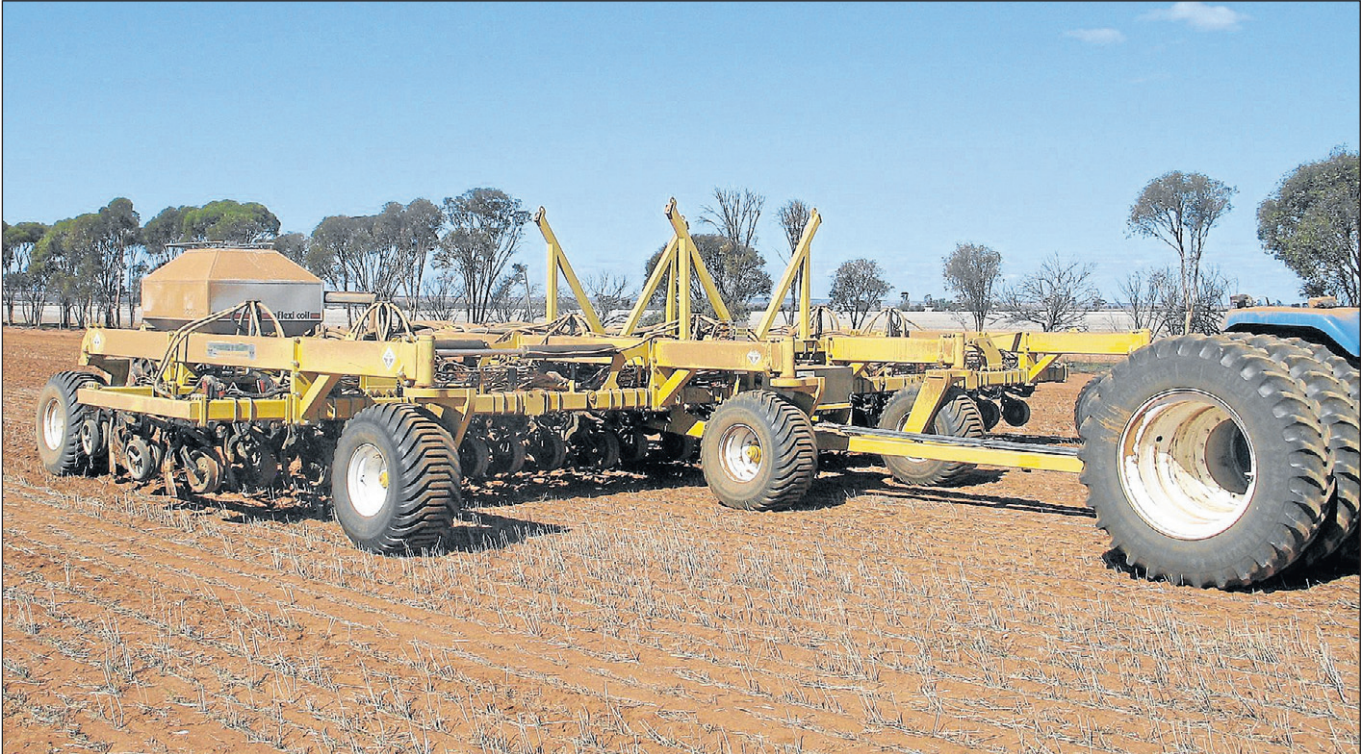
□ The beefy Moisture Manager weighs in at 25 tonnes but is easily carried by eight outrigger wheels boasting 600/55-22.5 flotation tyres. Weight is important in terms of penetrating tight soils.
